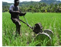
The Motorized Weeders for rice production (cut and bury) technology eliminate weeds in rice crops. The rotating blades of the weeders ensure effective weeding while minimizing damage to rice crops and soil. These machines can be used from the germination of rice plants until the canopy closes.
