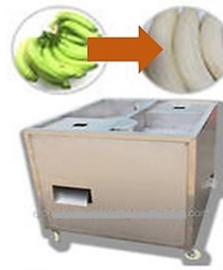
An industrial green banana peeler able to processes 600 units per hour
