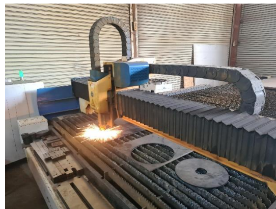
Figure 5: Laser Cutting of Metal Components for Grinders
