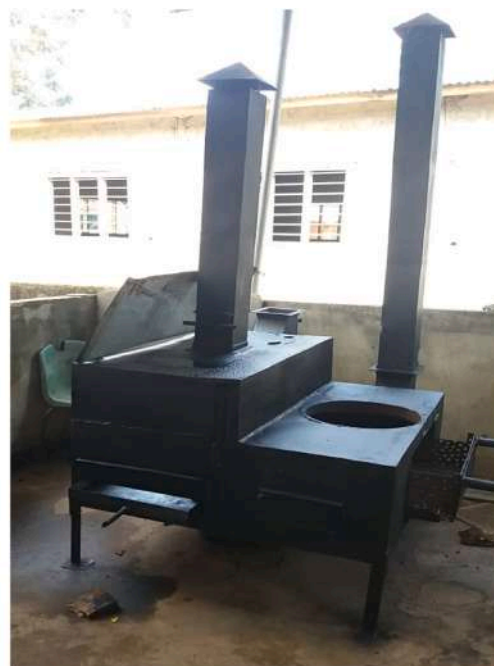
Fig. 3. Improved clay grill with two chambers (GA2C). (1): Grilling chamber; (2): Grid; (3): Combustion chamber; (4): Cover windows; (5): Chimney of grilling chamber; (6): Chimney of combustion chamber; (7): Dropped fat collection plate.
