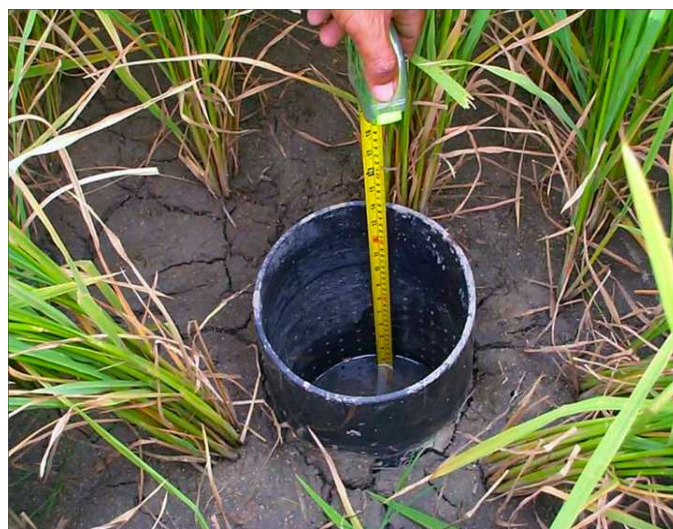
Figure 1. Field water tube used for observation of water levels by farmers. The ability to observe the level of the water table below the soil helps build confidence in AWD. (Photo: IRRI)
